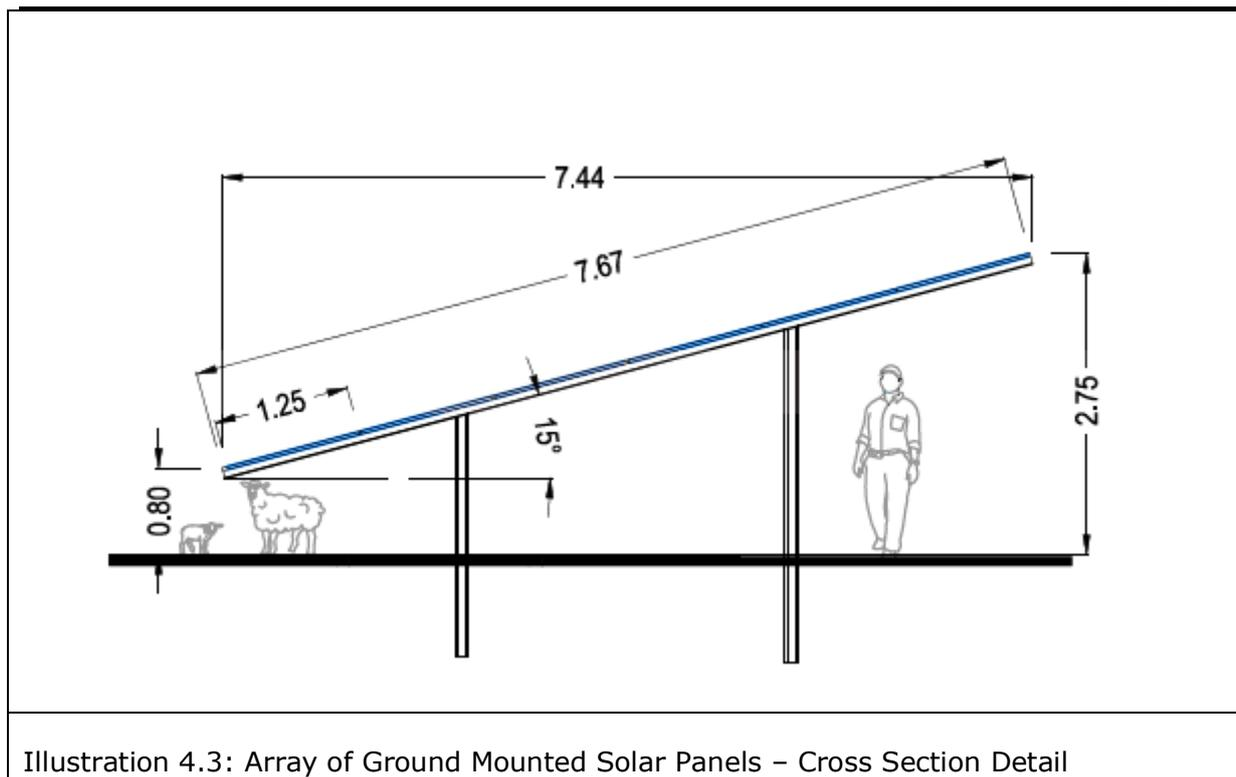
Illustration 4.3: Array of Ground Mounted Solar Panels – Cross Section Detail
