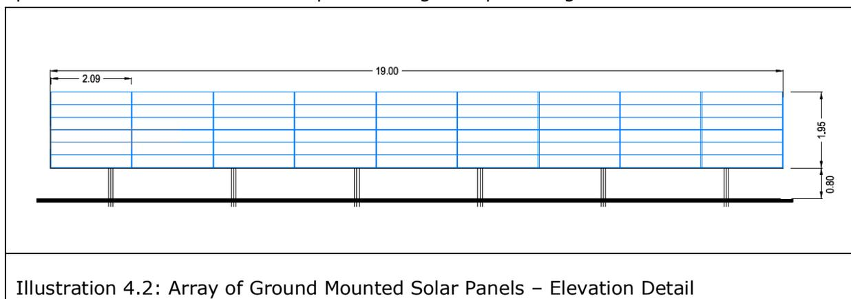
Illustration 4.2: Array of Ground Mounted Solar Panels – Elevation Detail
